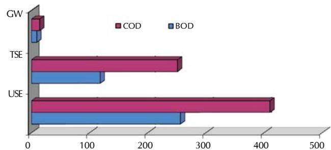
**Figure 3: Mean biological oxygen demand (BOD) and chemical oxygen demand (COD) of untreated (USE) and treated (TSE) sewage effluents in comparison to groundwater (GW)**
