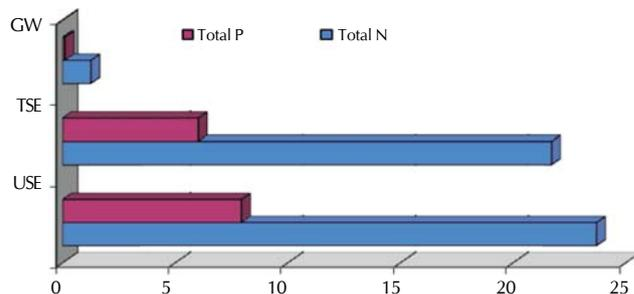
**Figure 5: Mean total N and total P of untreated (USE) and treated (TSE) sewage effluents in comparison to groundwater (GW)**
