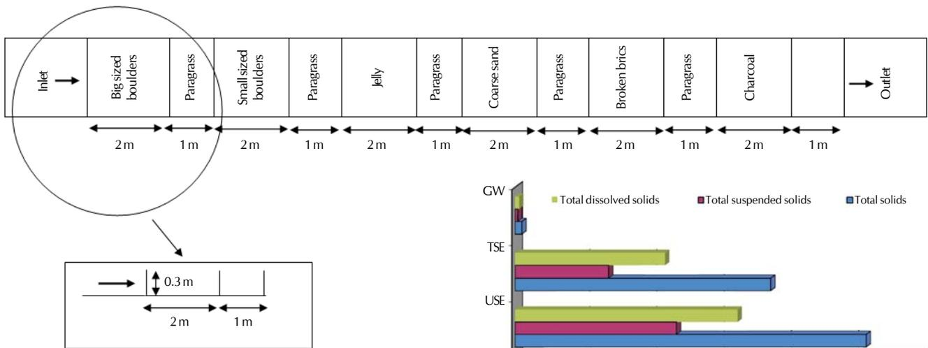
**Figure 1: Lay-out of constructed wetland components**
