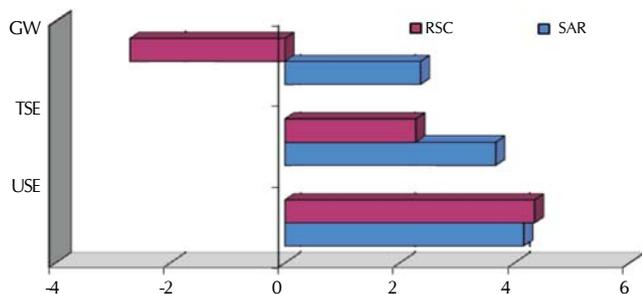
**Figure 4: Mean residual sodium carbonate (RSC) and sodium adsorption ratio (SAR) of untreated (USE) and treated (TSE) sewage effluents in comparison to groundwater (GW)**
