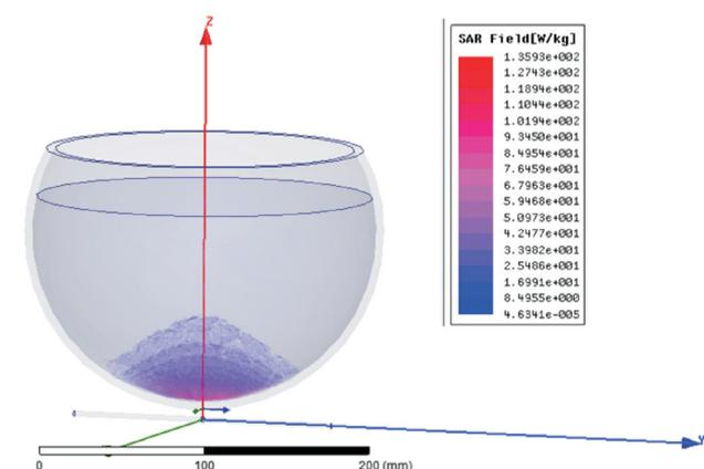
Figure 2: The human head one layer model along with SAR distribution. This human head model is taken in the HFSS simulation
