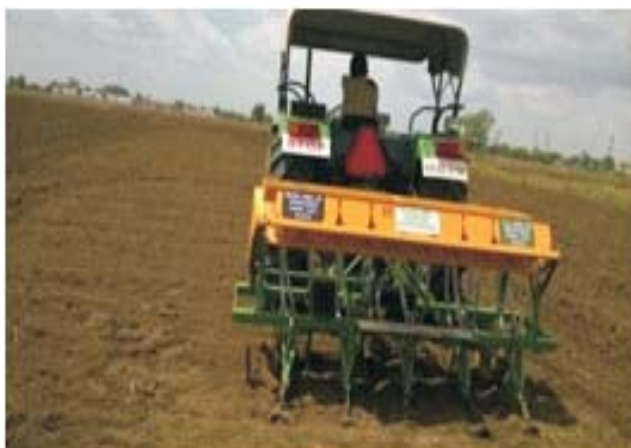
Figure 8: Field performance of inclined plate planter
